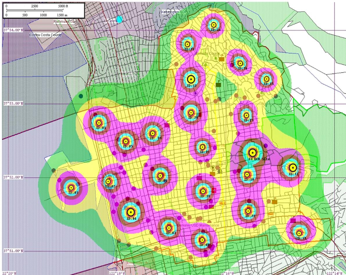
Sound intensities are shown as contours, the outermost is 70 – 75 dB.
